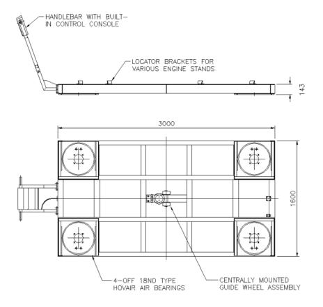
**Construction:** All steel construction, handlebars with built-in control console
