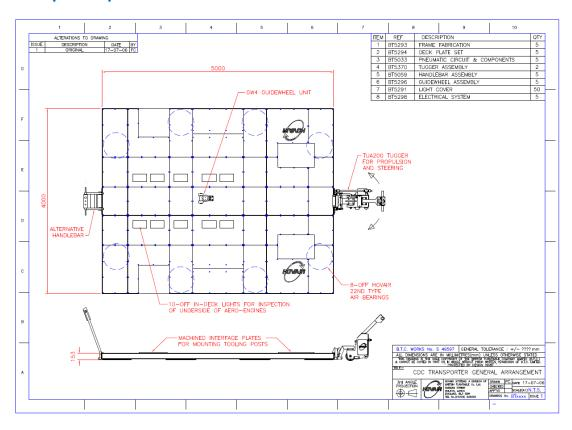
**Construction:** All steel construction, detachable handlebars with built-in control console, detachable powered tugger unit with built-in controls
